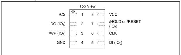
Figure 1b. W25Q64JW Pad Assignments, 8-pad WSON 6x5-mm/8x6, XSON 4x4-mm, USON 4X3-mm (Package Code ZP, ZE, XG, IIII)
