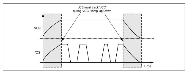
Figure 58b. Power-up, Power-Down Requirement
