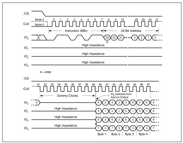
Figure 20. Fast Read Quad Output Instruction
