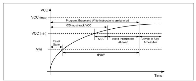
Figure 58a. Power-up Timing and Voltage Levels
