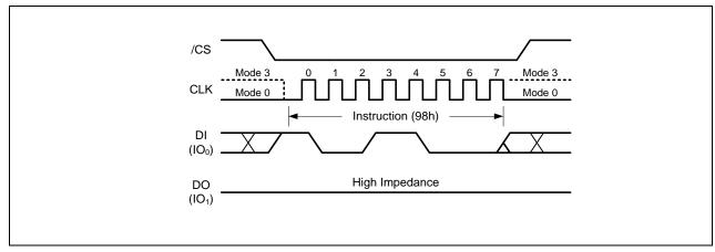
Figure 57. Global Block Unlock Instruction for SPI Mode
