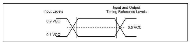
Figure 59. AC Measurement I/O Waveform
