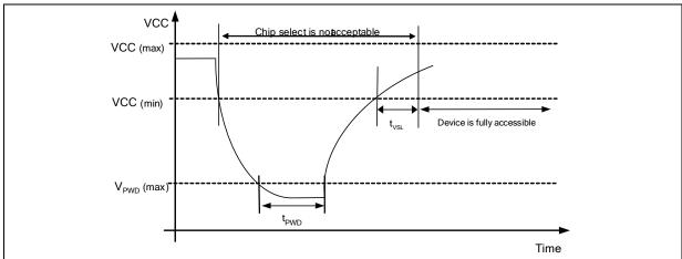
Figure 58c. Power Cycle Requirement
