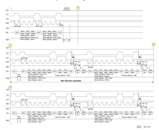
Figure 20: Multi plane cache read operation Timings
