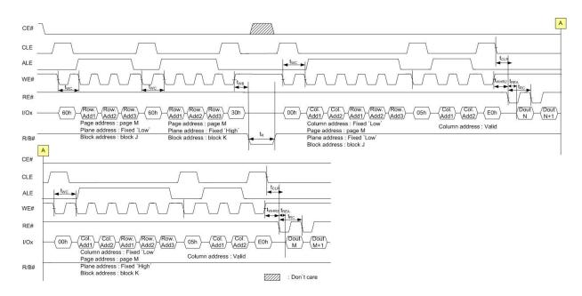
Figure 18: Multi plane page read operation timings with random data output
