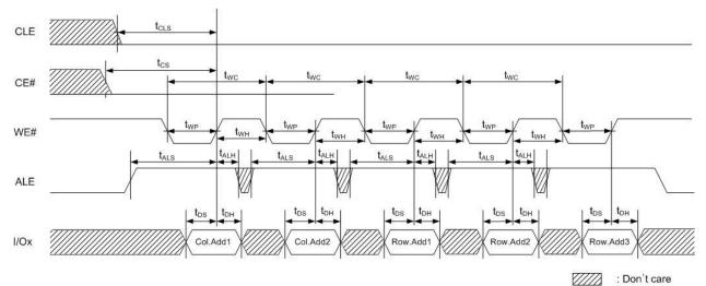
Figure 8: Address latch timings
