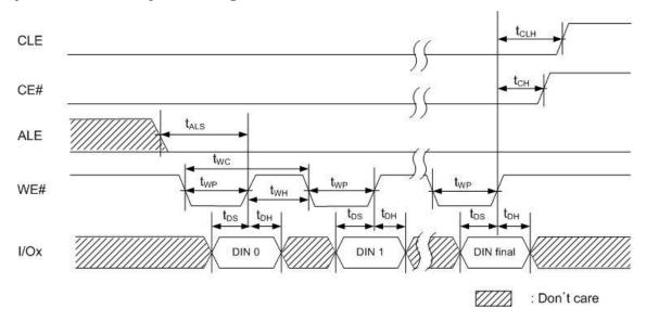
Figure 9: Input data cycle timings
