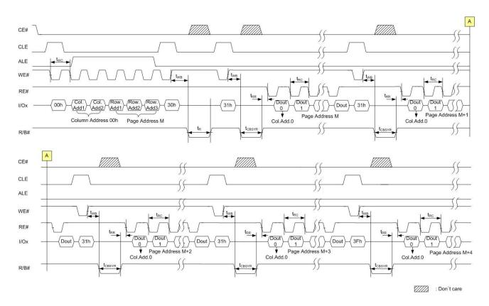
Figure 19: Cache read operation timings
