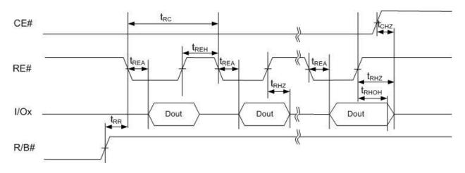
Figure 10 : Data output cycle timings
