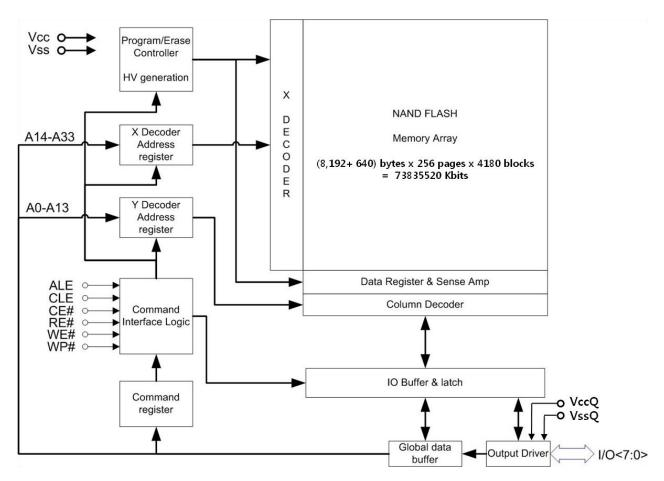
Figure 3: Block diagram(SDP)
