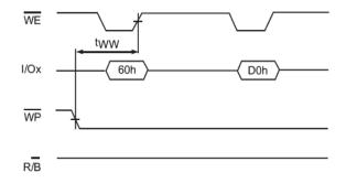
Figure 56: Enable Erasing
