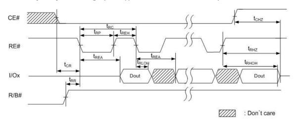
Figure 11: Data output cycle timings (EDO)
