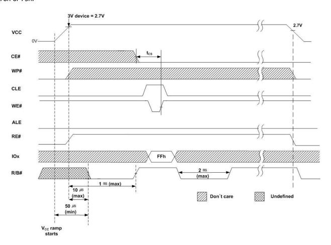
Figure 52: Data protection and power on / off
