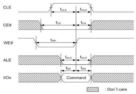
Figure 7: Command latch timings
