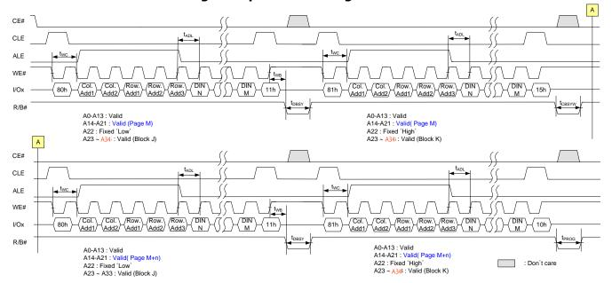
Figure 28: Multi plane cache program operation timings
