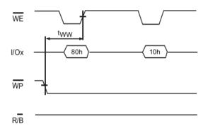
Figure 54: Enable Programming
