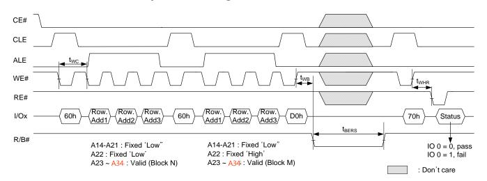
Figure 30: Multi plane erase operation timings
