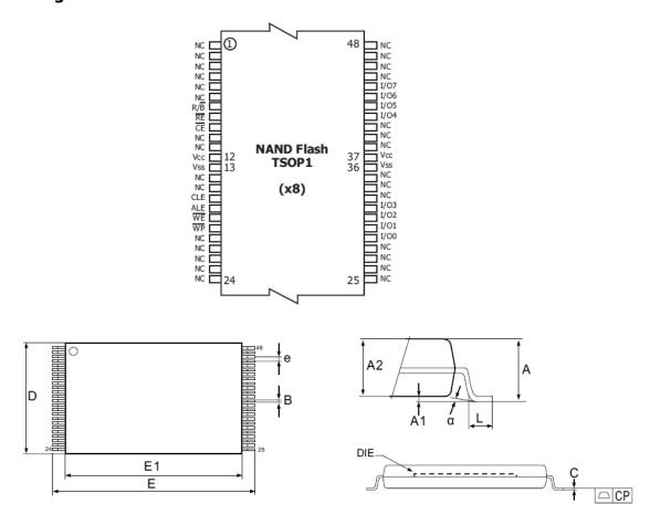
Figure 2: 48-pin TSOP
