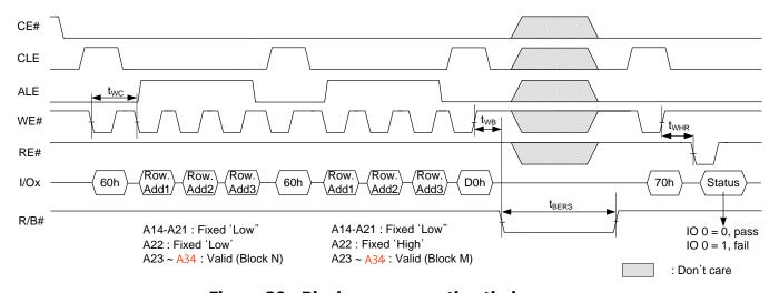
Figure 29: Block erase operation timings
