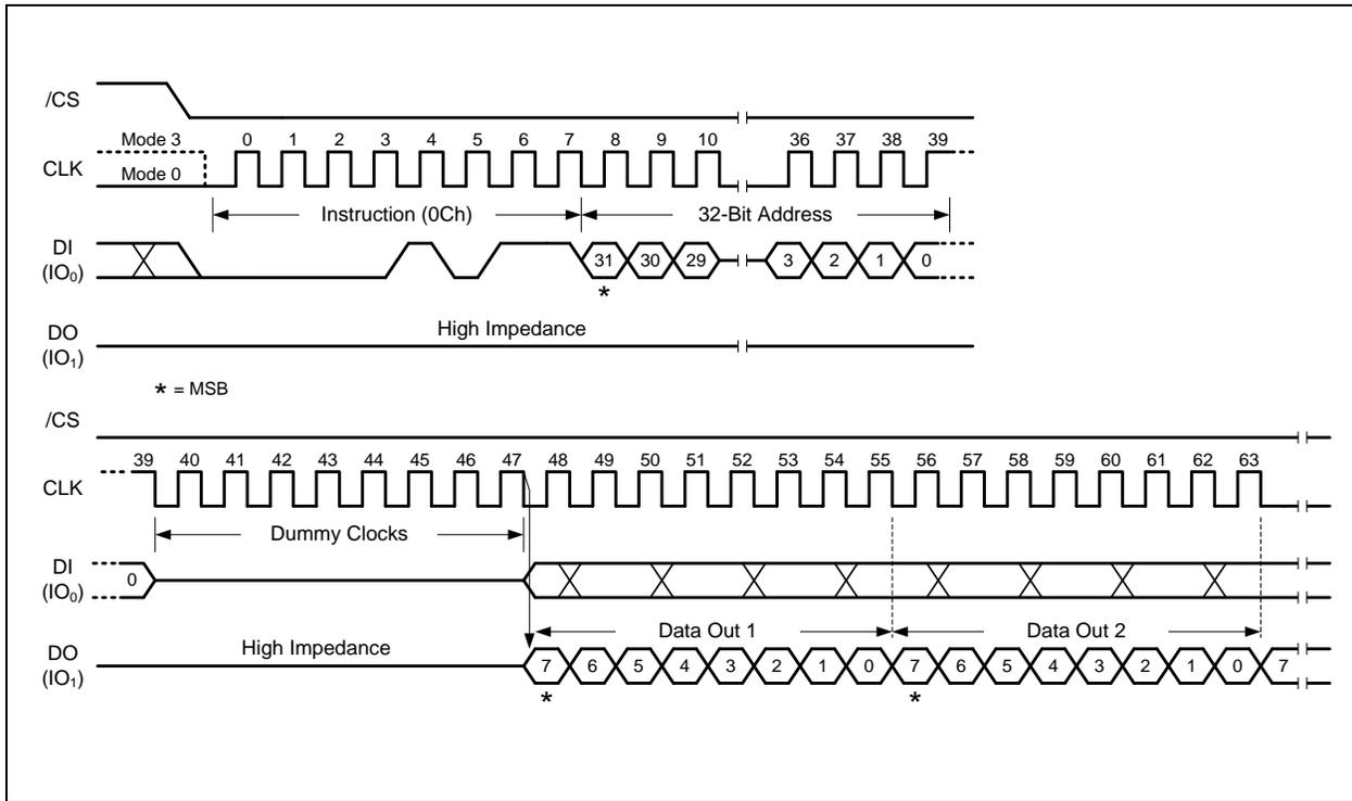
Figure 18. Fast Read with 4-Byte Address Instruction
