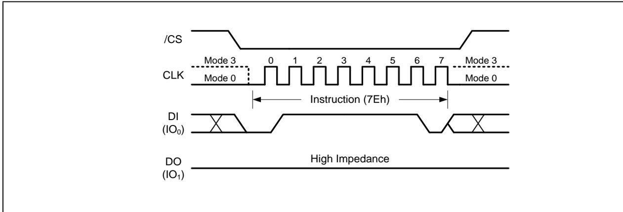
Figure 58. Global Block Lock Instruction for SPI
