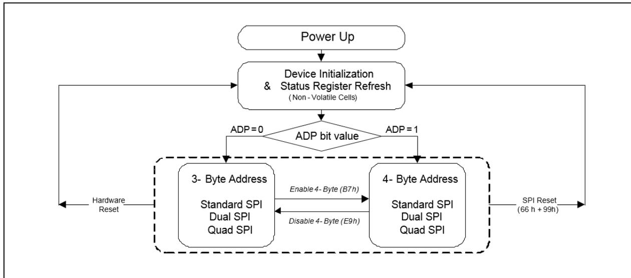
Figure 3. W25Q512JV Serial Flash Memory Operation Diagram
