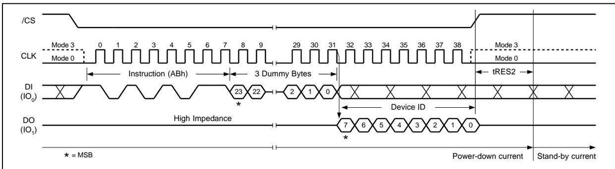
Figure 45b. Release Power-down / Device ID Instruction
