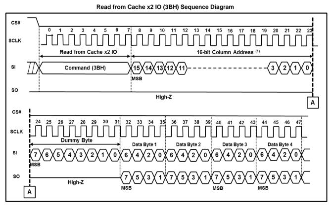
Note : 1 Page = 2K+64B, 16-bit column address consists of 4 wrap bits and 12 column address bits.
