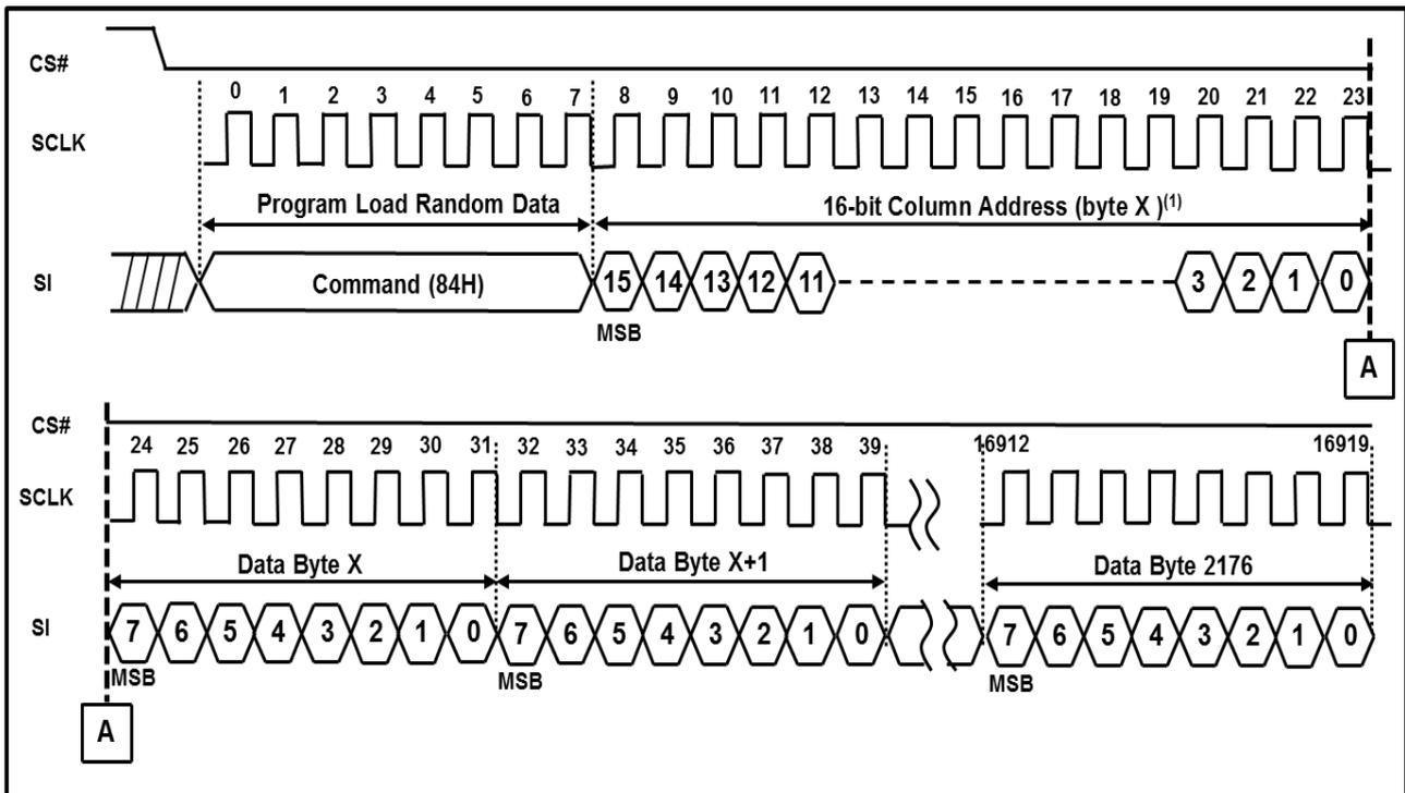
**Note : 1 Page = 2K+64B, 16-bit column address consists of 4 wrap bits and 12 column address bits.**
