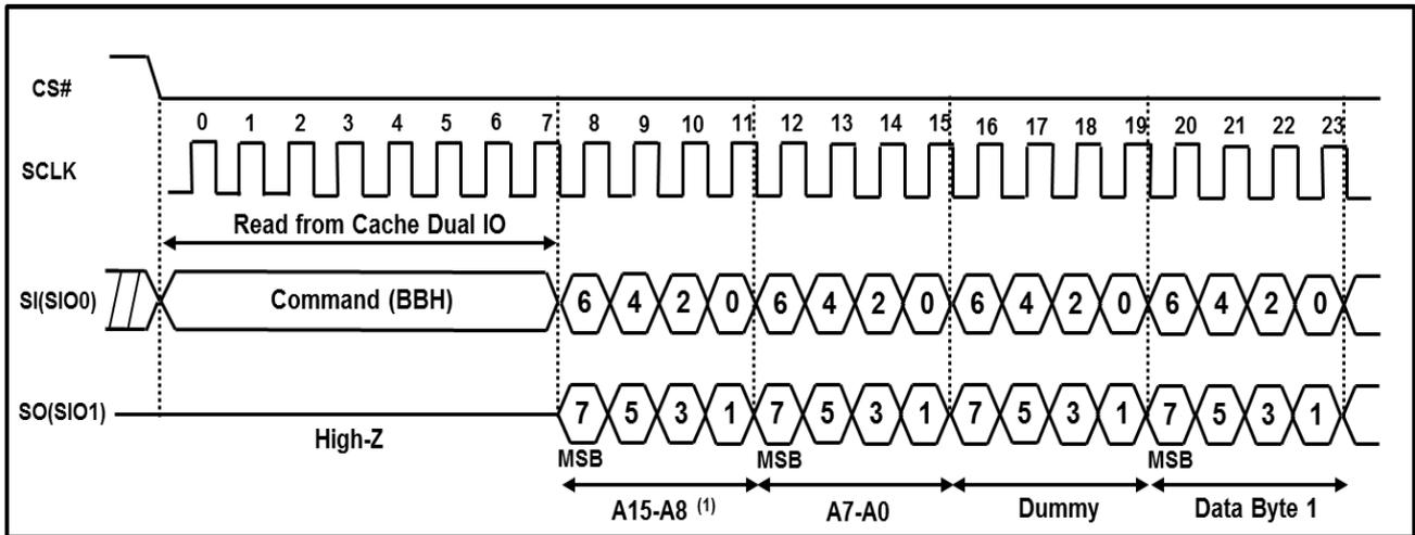
Note : 1 Page = 2K+64B, 16-bit column address consists of 4 wrap bits and 12 column address bits.
