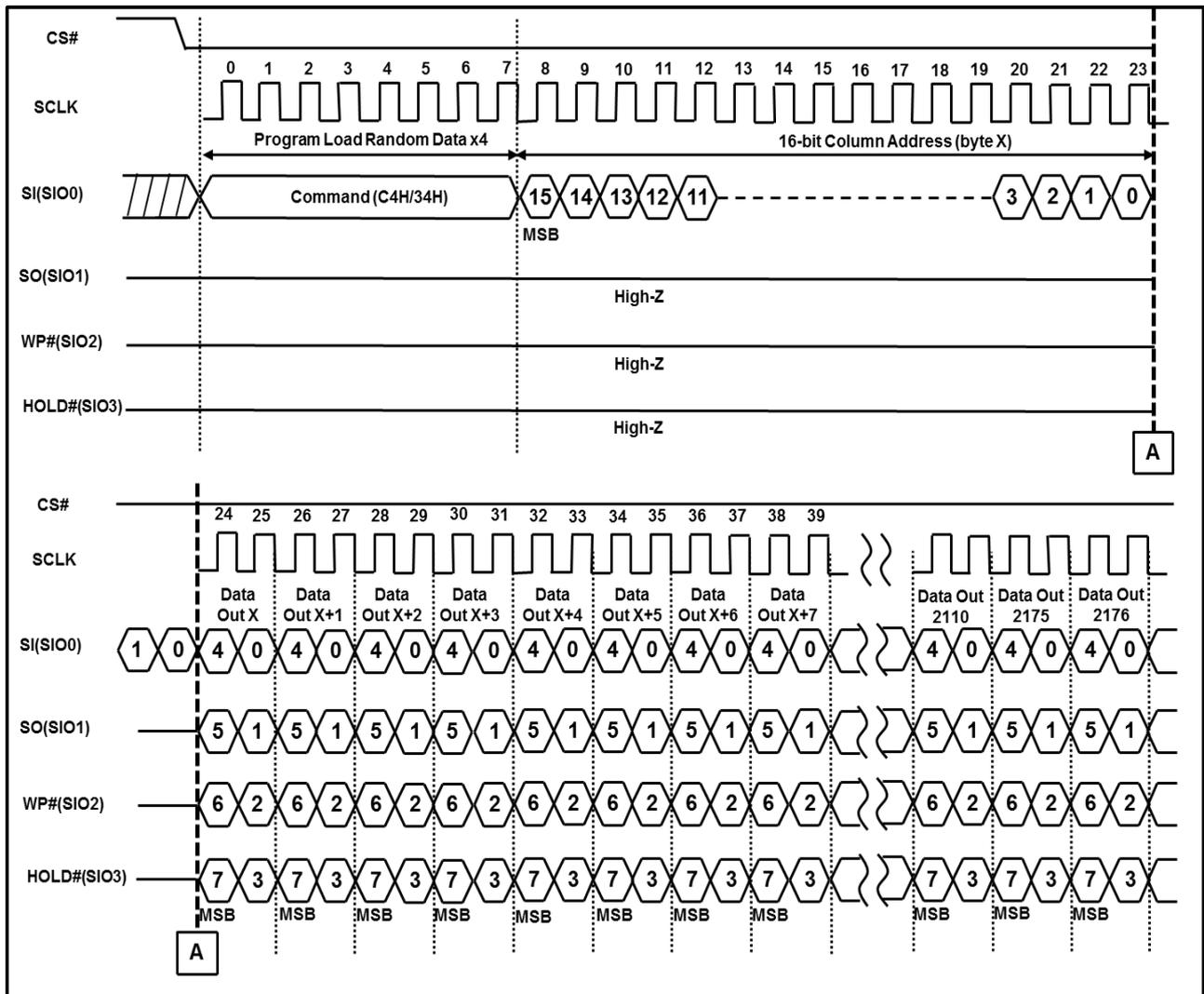
Note : 1 Page = 2K+64B, 16-bit column address consists of 4 wrap bits and 12 column address bits.
