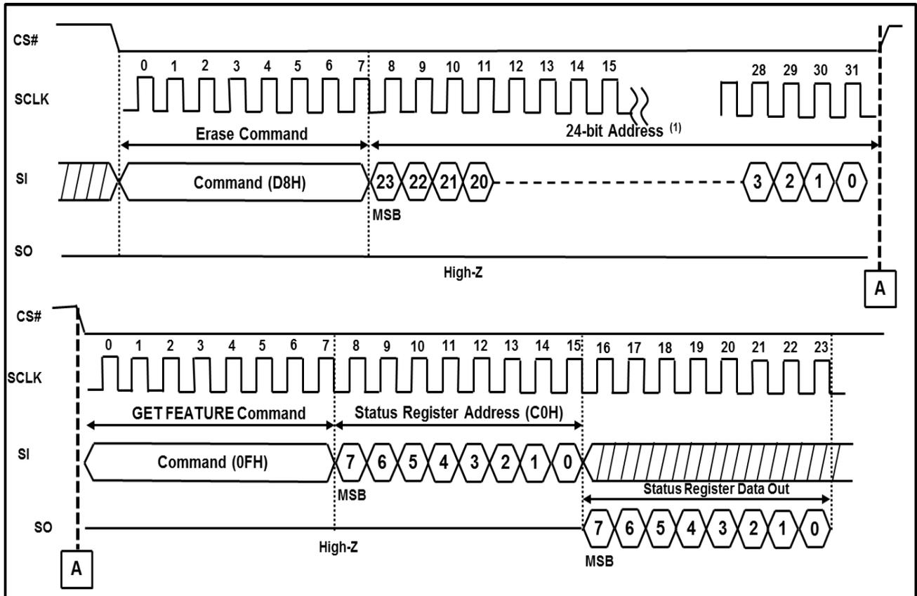
Note : If # of Block = 1024, 24-bit address consists of 8 dummy bits and 16 page/block address bits.
