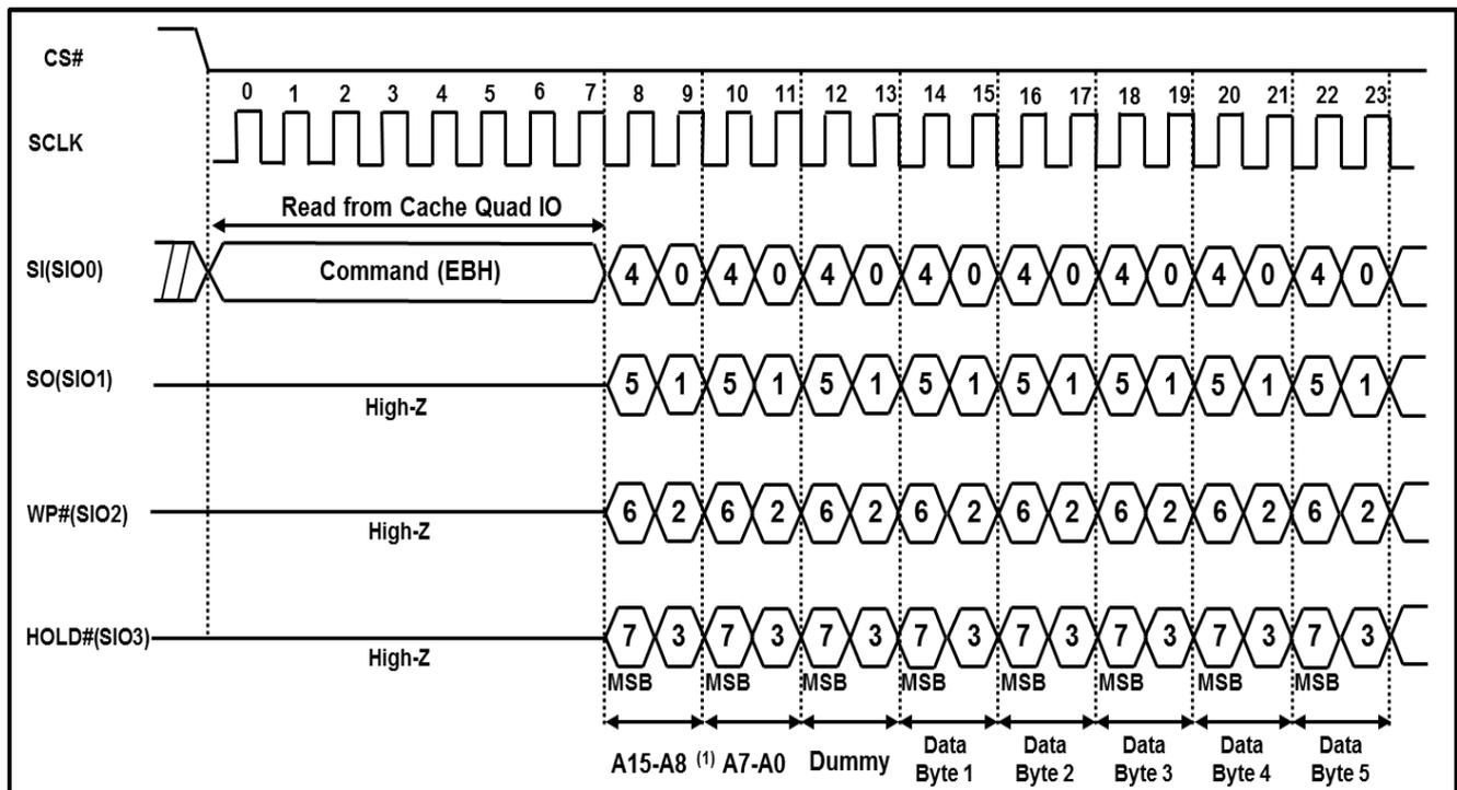
**Note : 1 Page = 2K+64B, 16-bit column address consists of 4 wrap bits and 12 column address bits.**
