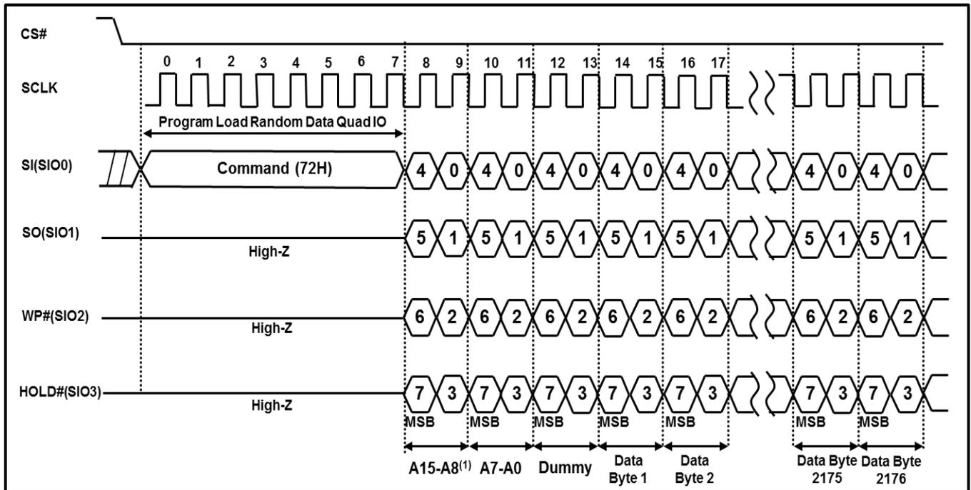
**Note :** 1 Page = 2K+64B, 16-bit column address consists of 4 wrap bits and 12 column address bits.
