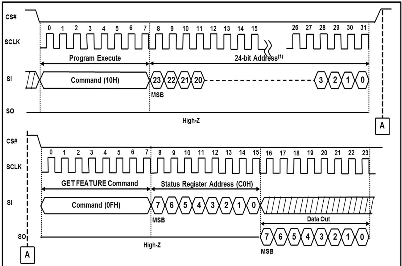
Note : If # of Block = 1024, 24-bit address consists of 8 dummy bits and 16 page/block address bits.
