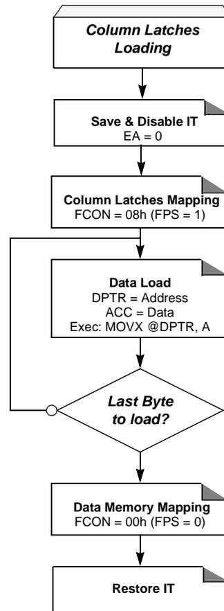
Note: 1. The last page address used when loading the column latch is the one used to select the page programming address.
