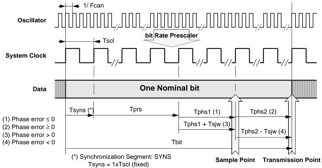
Tbit calculation:  $T_{\text{bit}} = T_{\text{syns}} + T_{\text{prs}} + T_{\text{phs1}} + T_{\text{phs2}}$
