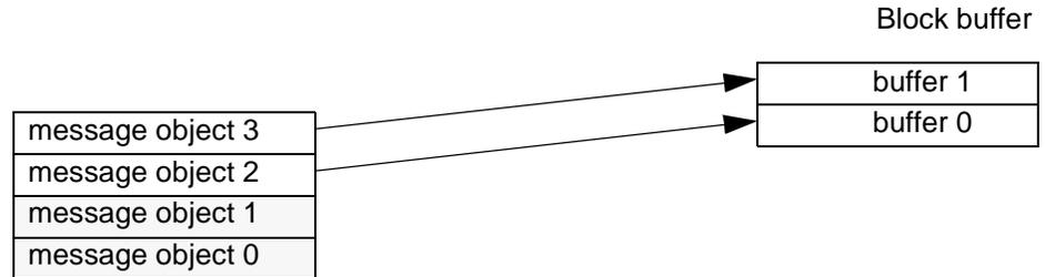
The same acceptance filter must be defined for each message objects of the buffer. When there is no mask on the identifier or the IDE, all messages are accepted.
