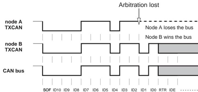
The CAN protocol handles bus accesses according to the concept called "Carrier Sense Multiple Access with Arbitration on Message Priority".
