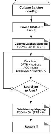
Note: 1. The last page address used when loading the column latch is the one used to select the page programming address.
