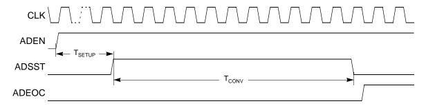
Note: Tsetup min, see the AC Parameter for A/D conversion.
