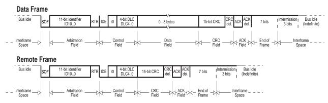
A message in the CAN standard frame format begins with the "Start Of Frame (SOF)", this is followed by the "Arbitration field" which consist of the identifier and the "Remote Transmission Request (RTR)" bit used to distinguish between the data frame and the data request frame called remote frame. The following "Control field" contains the "IDentifier Extension (IDE)" bit and the "Data Length Code (DLC)" used to indicate the
