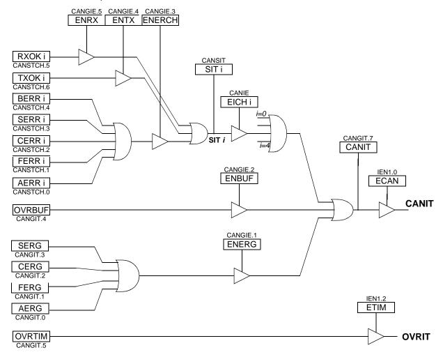
To enable a transmission interrupt:
