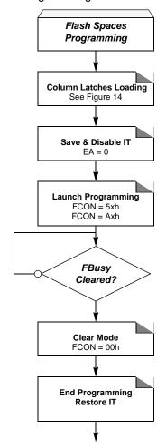
Figure 15. Flash and Extra row Programming Procedure
